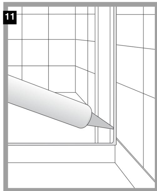
**DO NOT USE THE SHOWER ENCLOSURE FOR 24 HOURS TO ENSURE SILICONE IS FULLY CURED AND WATERPROOF.**
